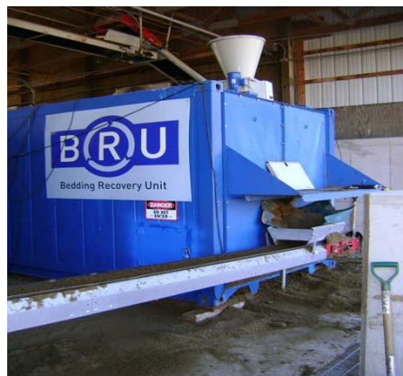
Bedding Recovery Unit
