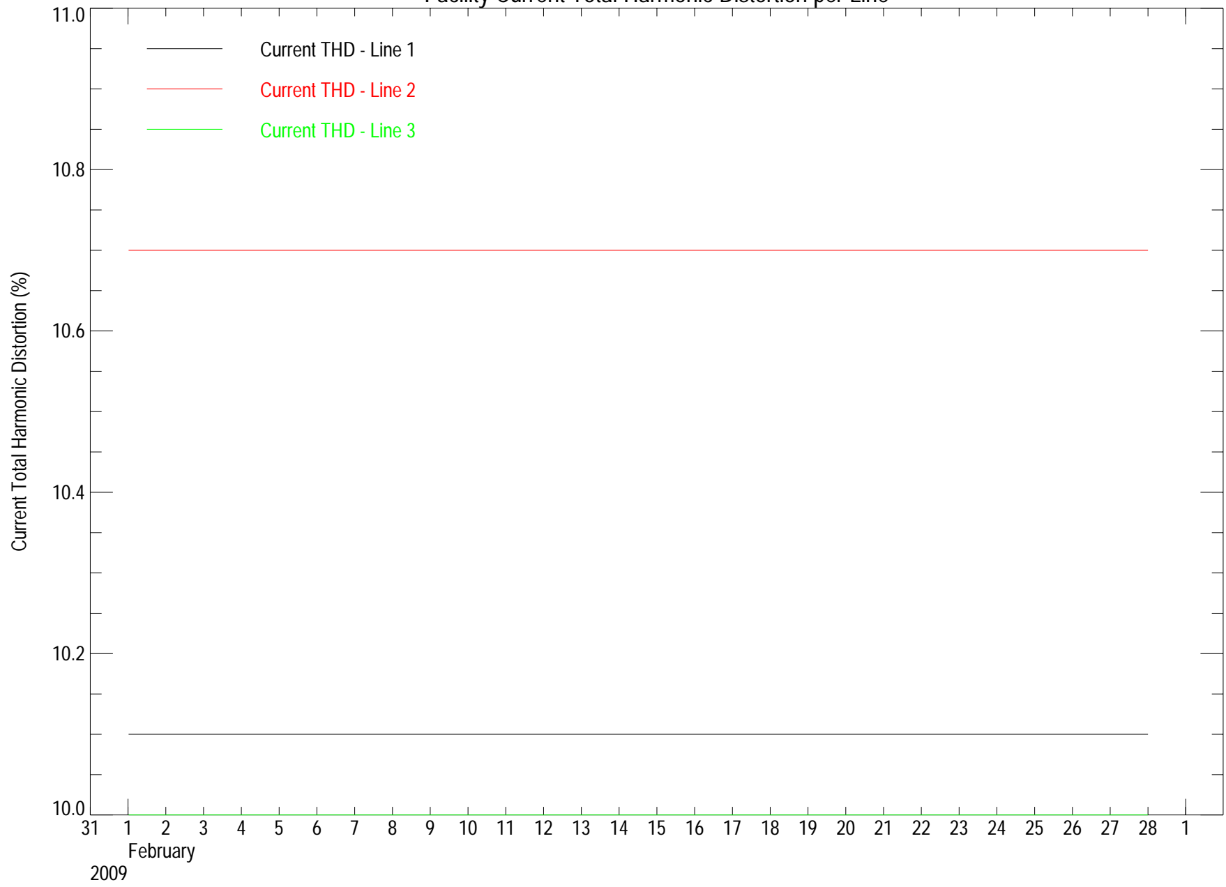
Facility Current Total Harmonic Distortion per Line
